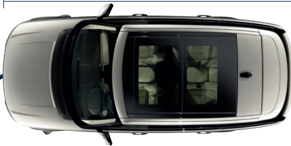
Standard Overall length 4,999mm (Long Wheelbase 5,199mm)
