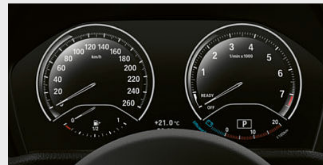
The hybrid-specific instrument cluster informs you about all relevant data relating to the innovative plug-in hybrid drive. With the hybrid-specific instrument cluster, you always have all the relevant information about the innovative plug-in hybrid drive at your fingertips. For example, you can read the output display of the electric motor as well as the charge level indicator and the purely electric and combined range.
