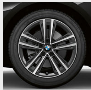
□ 17" light alloy wheels Double-spoke style 548 Bicolour Orbit Grey metallic, gloss-lathed, wheel size 7.5J x 17 with 225/45 R17 tyres.
