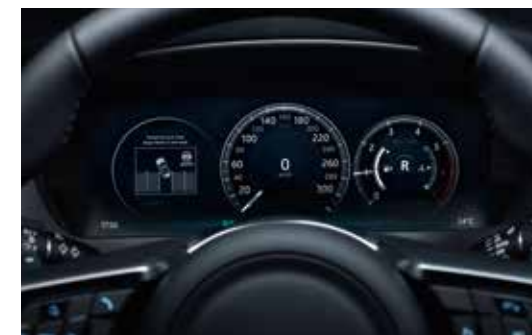
12.3 inch Instrument Panel Display with virtual dials
