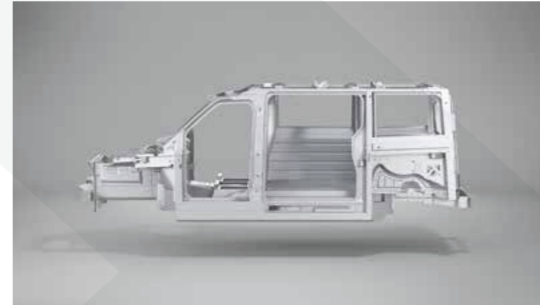
Built using anodised, bonded aluminium, an advanced production technique adopted from the aerospace and motorsport industries.
