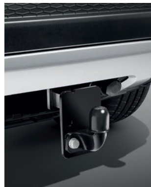
Multi-Height Tow Bar and Armature VPLWT0159 and either VPLWB0139, VPLWB0136 or VPLWB0137
